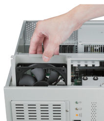
Easy-to-maintain cooling fan
