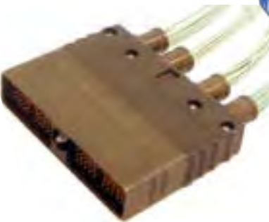
4 modules metallic plug, with cadmium plating, fitted with cabled modules, a backshell and 4 chimneys.
