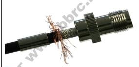
**6.** Insert the so prepared cable end into the connector housing as far it goes (click).
