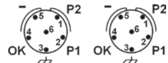
Pin-out for the 2 power connectors of the Ring and managed models
