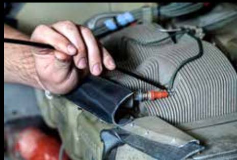
Inspecting cylinder in aircraft motor with VSA2-1M
