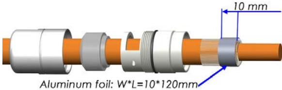
Step 4: Wrap foil over braided shielding
