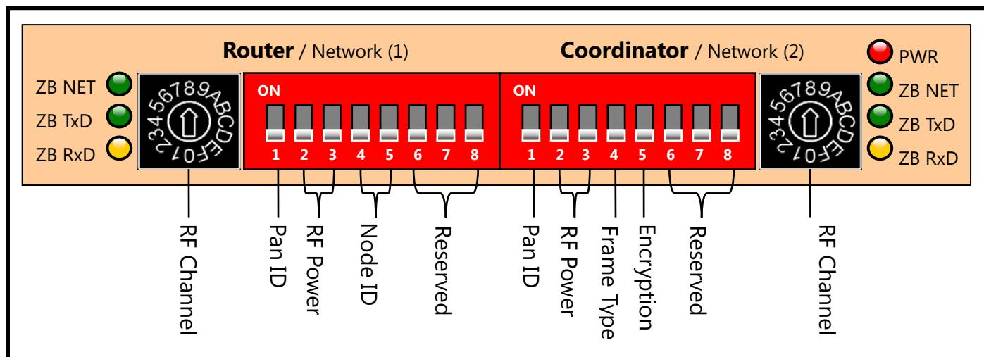
After configuration, user can confirm the connection and communication quality via the state of LED indicators. Please refer the table as below.
