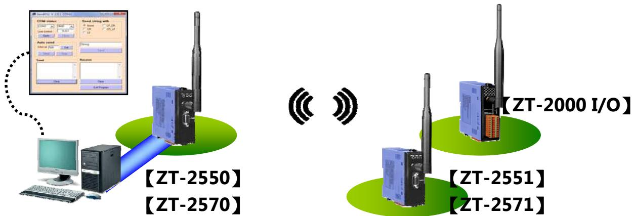
2. Set the Pan ID/ Node ID/ RF Channel/ RF Power for the Router / Network (1) via the hardware rotary dip switches to be consistent with the original coordinator (ZT-2550/ZT-2570). Note that the Node ID should be unique in the first network.
