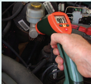
Laser pointer identifies target area.
